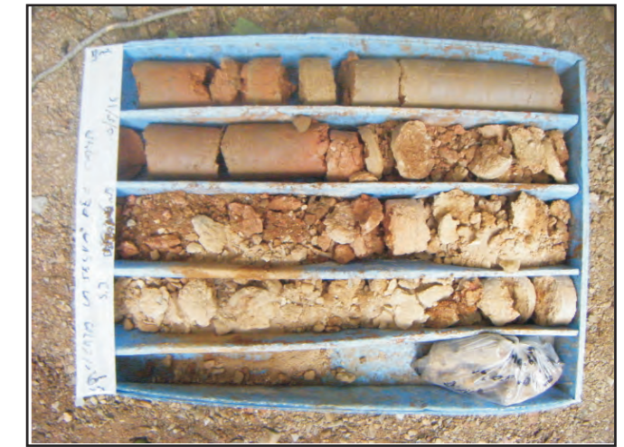
Sondeig S-3. Caixa 3,0 a 6,0 m
