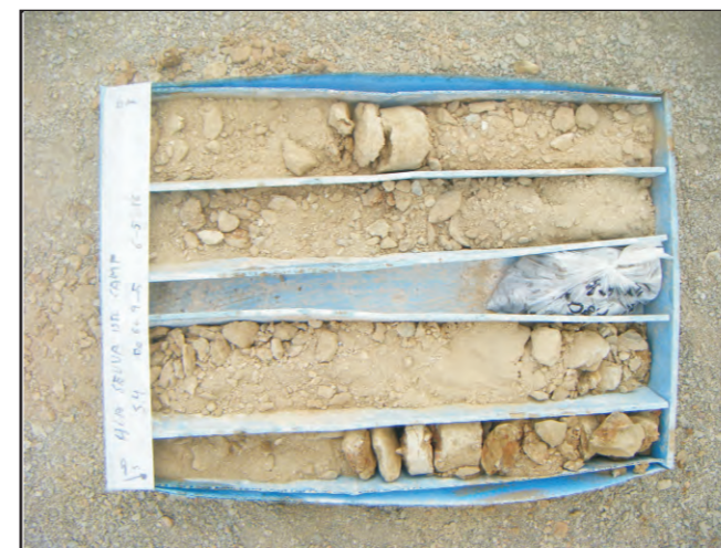
Sondeig S-3. Caixa 6,0 a 9,0 m
