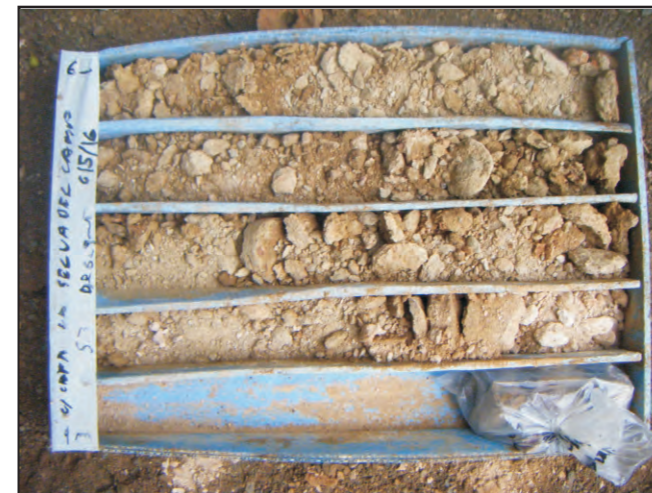
Sondeig S-3. Caixa 6,0 a 9,0 m
