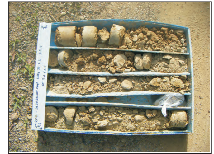
Sondeig S-2. Caixa 3,0 a 6,0 m
