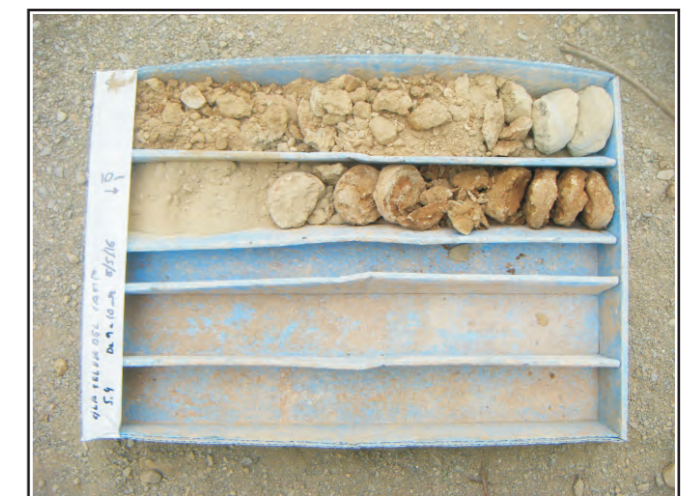
Sondeig S-3. Caixa 9,0 a 10,0 m
